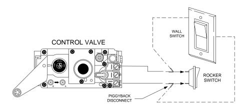
Remember the Rocker Switch must be turned to "OFF" while using the Wall Switch.
